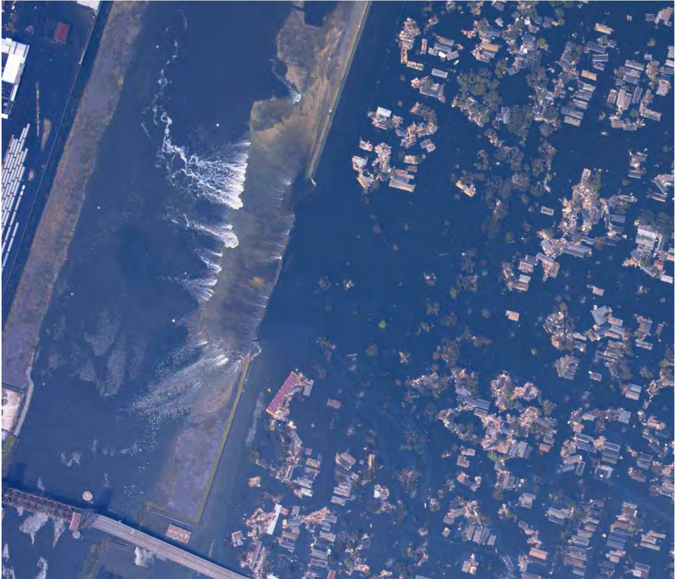
Fig. 4.3: Airborne digital imagery of the south breach at the Lower Ninth Ward. Water is shown flowing back into the IHNC. (courtesy NOAA, August 31, 2005).
