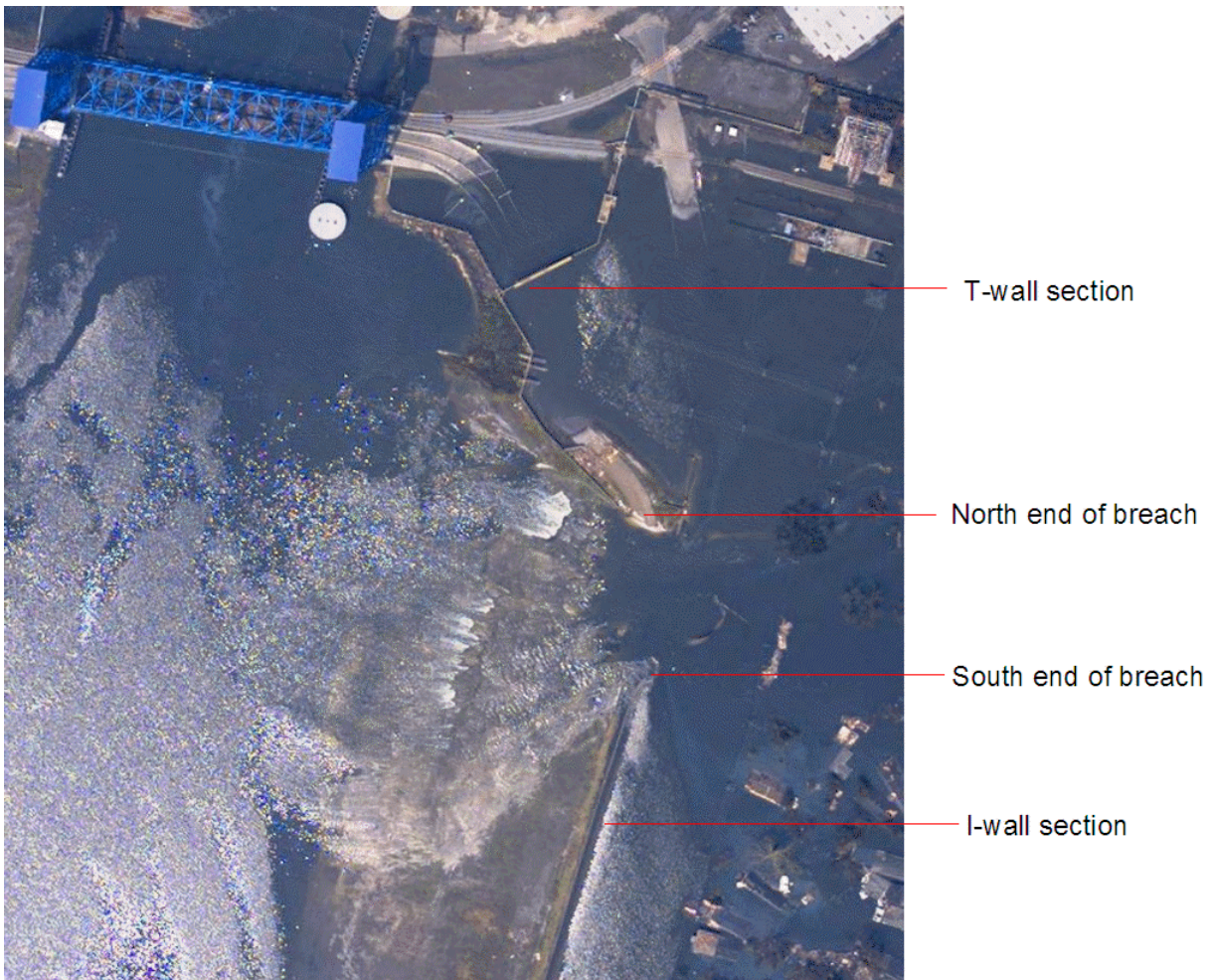
Fig. 4.7, Airborne digital imagery of the north breach at the Lower Ninth Ward. Water is shown flowing back into the IHNC. (courtesy NOAA, August 31, 2005).
